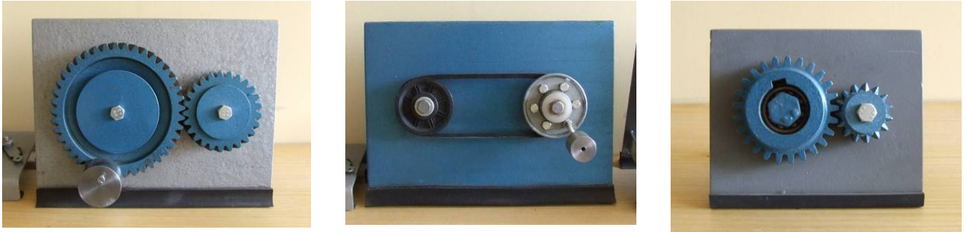
Figure 9. Transmission and reduction gears: rotation lasted 1 - 2.5 sec.
