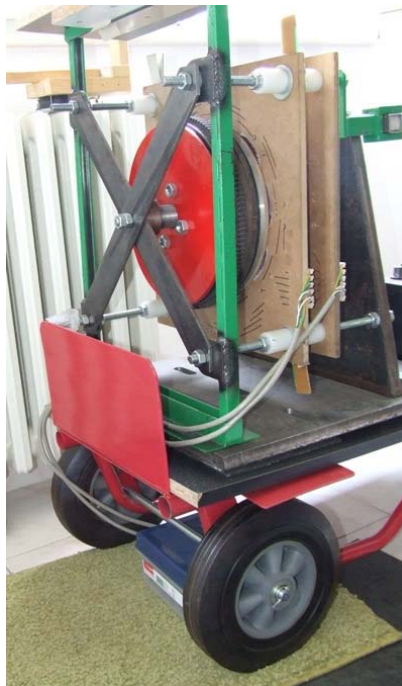
Figure 10. Flywheel with mass of 20 kg: rotation lasted 1 min. - 1 min. 12 sec.
